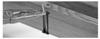
40 Close the top lid and carefully strike the plunger pin as to make a noticeable mark in the top. This will serve as the location for the steel tack.
