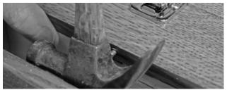
Locate the tack mark made in the top and hammer tack into the rail. Make sure the top is being supported on the workbench as not to bend the hinges.
