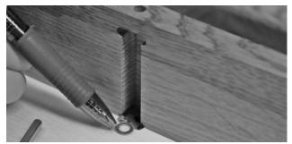
**39** Using a pair of needle nose pliers, push the end of the pin through the bottom washer and release it through the top hole. This can be a bit awkward and challenging so several attempts might be necessary. Scan the QR code above to see a video of this process.
