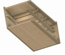
Install remaining chest side as shown, It will be a little challenging to get all of the parts in their proper grooves. Take your time and ensure all edges are flush and construction is correct.
