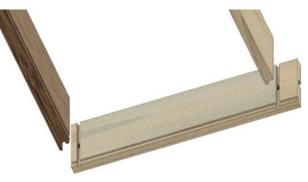
21 Slide the 1/8" thick plywood drawer bottom into the drawer as shown. The drawer bottom can be glued into place or float without being glued into the drawer.
