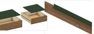
After all felt has been installed, let the chest sit open for a few hours to dry.
