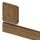
Slide raised panel into lid assembly making sure the raised panel profile shows to the front. Make sure the end rails set flush on the outside edges.
