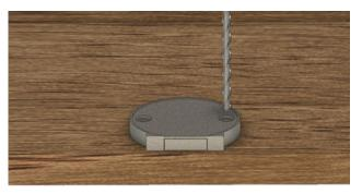
Be careful to not drill through wood. CAUTION: Do not mount or drill lock on front face of lid.
