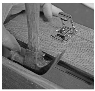
Locate the tack mark made in the top and hammer tack into the rail. Make sure the top is being supported on the workbench as not to bend the hinges.
