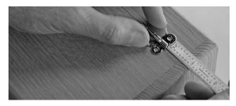
Mark the position of the hinge screws.
