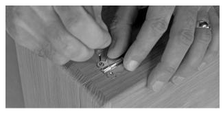
Drill all the hardware screw holes with a 3/32" drill bit (excluding the top lid tack).
